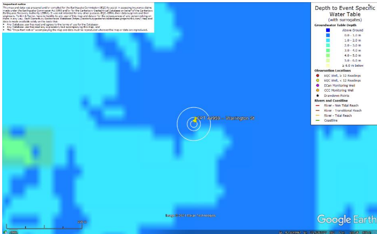
Figure 73: Depth to groundwater table for Jun-11 EQ.
