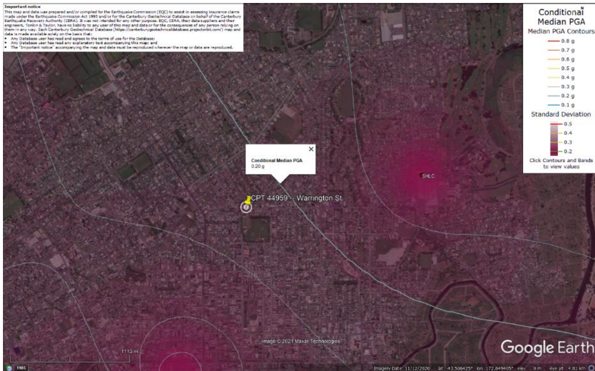
Figure 67: PGA for Sep-10 EQ (st. dev. = 0.300-0.325 ln units).
