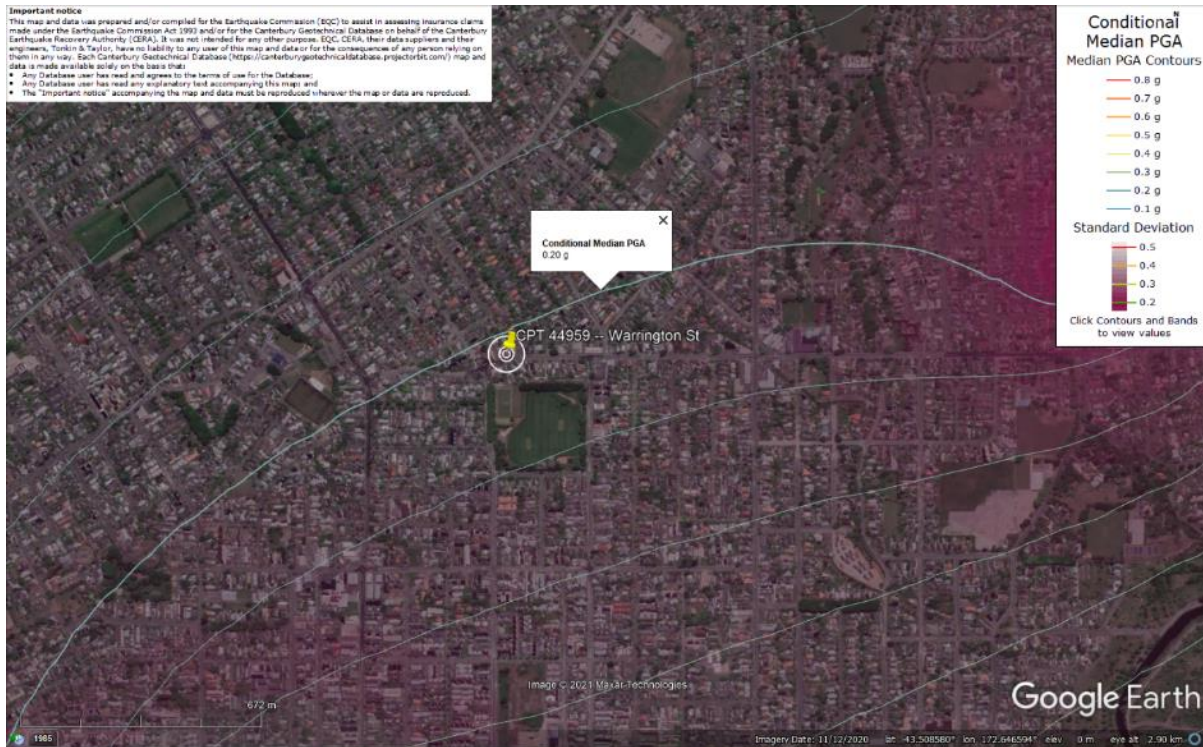
Figure 69: PGA for Jun-11 EQ (st. dev. = 0.350-0.375 ln units).
