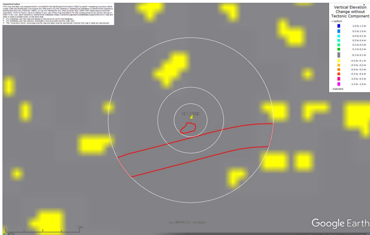
Figure 24: Ground surface subsidence without tectonic component for Jun 2011 Earthquake according to the LiDAR DEM.
