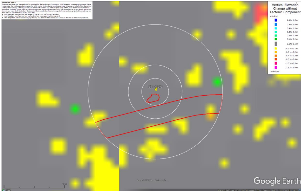
Figure 25: Ground surface subsidence without tectonic component for Dec 2011 Earthquake according to the LiDAR DEM.
